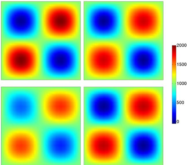
**Fig. 6.** Reconstruction of basal sliding coefficient  $\beta$  from noisy synthetic observations ( $\text{SNR} = 100$ ) from Model III. Shown are the truth  $\beta$  field (top left) and the reconstruction for  $L = 10$  with linear rheology (top right) and with nonlinear rheology (bottom left). The bottom right image shows the reconstruction for a nonlinear rheology with  $L = 40$ .
