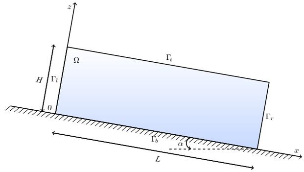
**Fig. 2.** Coordinate system and cross section through a three-dimensional slab of ice as used in the computational experiments.
