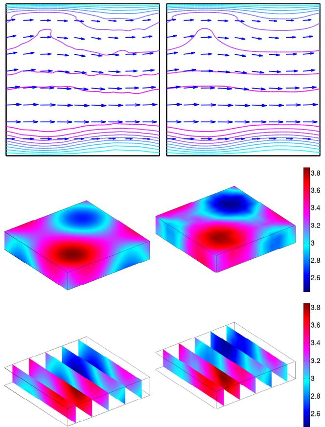
**Fig. 7.** Reconstruction of  $n$  exponent field in Glen’s flow law in Model IV. Noisy synthetic observations of the surface velocity (top left) are contrasted with the velocity field corresponding to the reconstructed  $n$  field (top right). The center and bottom rows show the truth (left) and reconstructed (right)  $n$  parameter fields.
